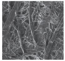
Cellulose filter media photo from scanning electron microscope of times.
