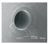
Close-up of work fuel injector needle seat.
