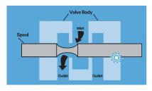
back and forth in the valve body, diverting oil to one side of the valve or the other. This type of value is typical in engine oil control circuits. If a particle lodges between the spool and valve body, it will erode small flakes from the metal surfaces. As these flakes are moved back and forth by the action of the spool, they can roll into a burr that jams the spool and disables the valve.
