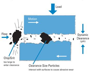
engine operation. The circuit actually generates additional particles as the fluid comes into contact with the precision machined surfaces of cyclinder walls and pistons, injector needles and pistons and crankshaft bearings. Contaminant levels can keep doubling with every new particle generated. The result can be catastrophic if these contaminants are not properly filtered out of the system.
