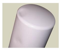
Dents in a steel filter canister create a concentration of stress, making the canister more susceptible to fatigue.
