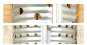
Liners with open holes can cause media tears during pleat movement.
