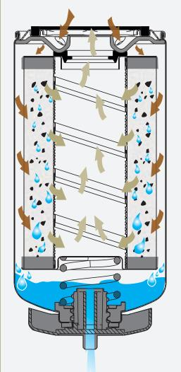
Clean fuel enters the filter through holes in the baffle/thread plate.
