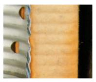
Donaldson cures its filter media (on left) before the filter is assembled, as shown by the consistent color of the entire surface of the filter media. The uneven color variation of the filter media of competitive brands (on right) is an indication that the filter media was cured after filter assembly.
