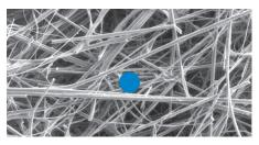
The microscopic image of Synteq lube filter media shows the consistency in fiber size and composition. The black circle in the picture above represents the diameter of a 20 micron particle easily captured by the media.
