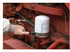
To avoid crossthreading DO NOT OVER TIGHTEN OR RETIGHTEN a filter.
