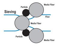
The fourth method of capture is called sieving and is the most common mechanism in liquid filtration. As shown at right, this is when the particle is too large to fit between the fiber spaces.
